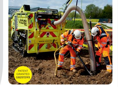
Powerful, towable, and compact (1m³) tracked VAC-EX unit with optional manual hose support arm.
